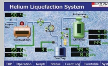
Control panel screen of the liquefaction system
