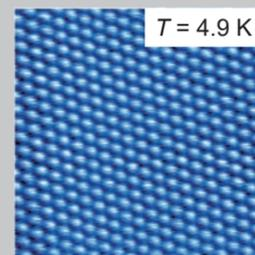
The first atomic-resolution STM image from the prototype system (April 2019)
