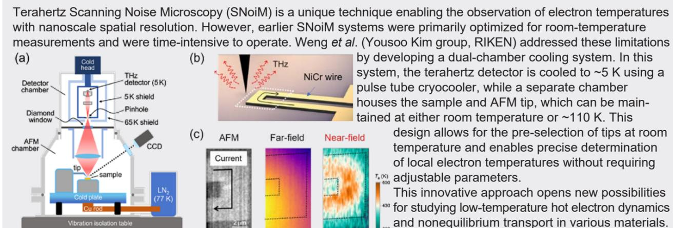
**Figure** (a) Schematic diagram of Cryo-SNoiM. (b) Diagram of hot electron imaging of NiCr wire. (c) Simultaneously obtained 2D images of the NiCr wire: topography, far-field and near-field (SNoiM) signals.
