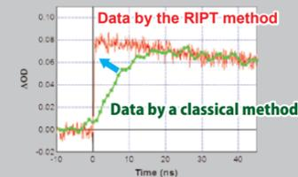
**Fig-2** Solved the problem of fluorescence contamination (Early Data)
