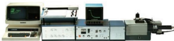
Gas-pressure based stopped-flow spectroscopy system
