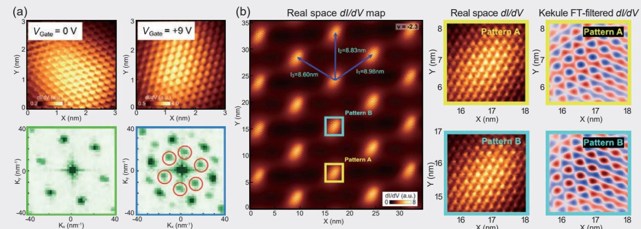
**Figure (a)**  $dI/dV$  map at  $V_{\text{Gate}} = 0 \text{ V}$ ,  $+9 \text{ V}$  and its Fourier-transformed image showing  $V_{\text{Gate}}$  dependent Kekulé order on MATTG. **(b)** Evidence of moiré translation symmetry breaking. (Left) Large-scale  $dI/dV$  map including 20 moiré AAA sites. (Right) Kekulé order in Pattern A and B in the left image, showing inverted contrast between neighboring AAA sites.
