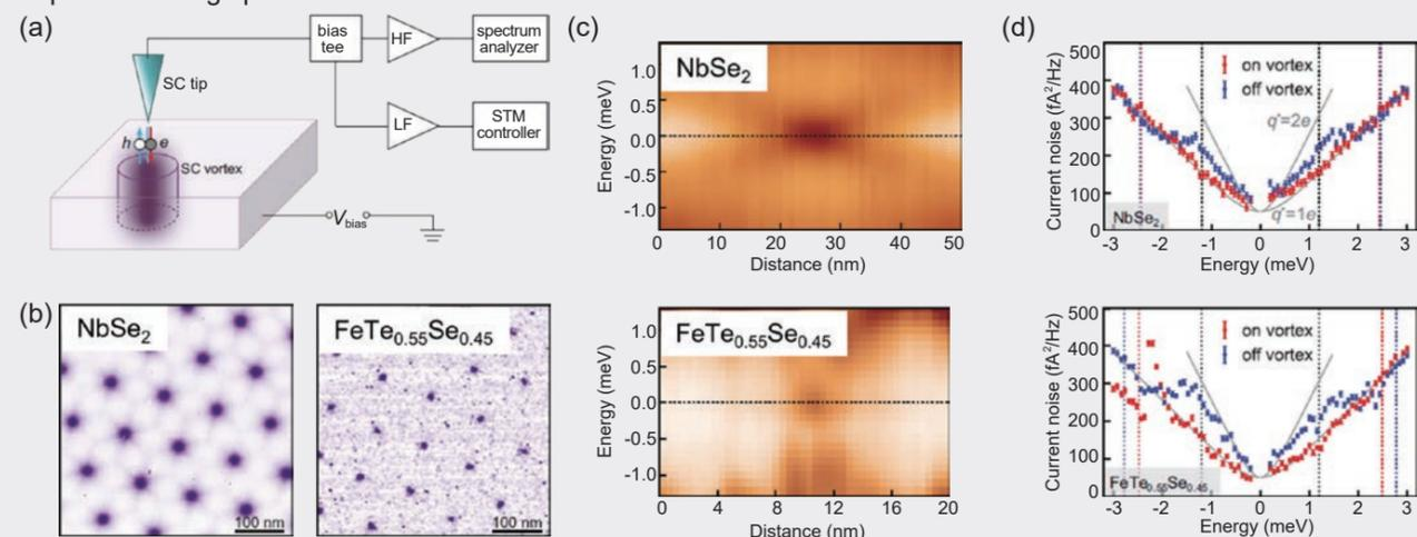
**Figure** (a) Scanning tunneling noise microscopy setup. (b) Vortex lattice image of NbSe<sub>2</sub> and FeTe<sub>0.55</sub>Se<sub>0.45</sub>. (c) Local DOS across the vortex core in NbSe<sub>2</sub> (splitting) and FeTe<sub>0.55</sub>Se<sub>0.45</sub> (no-splitting). (d) Local noise spectroscopy on and off vortices in NbSe<sub>2</sub> and FeTe<sub>0.55</sub>Se<sub>0.45</sub>.
