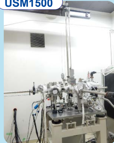
Photograph of the USM1500 system with the load lock, sample preparation, and measurement chambers
