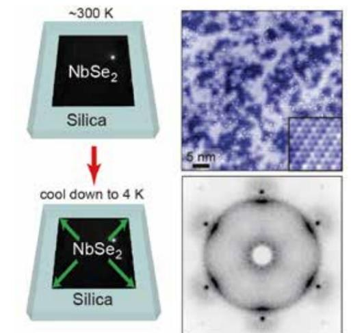
Strain manipulation of a charge density wave in  $\text{NbSe}_2$ . STM topograph (top right) and a Fourier transform of a  $dI/dV$  map showing quasiparticle interference (bottom right) [Gao *et al.*, *PNAS* (2018).]
