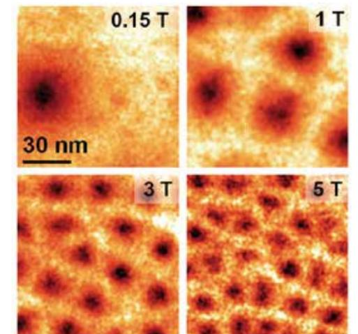
$dI/dV$  maps showing a vortex lattice on the surface of proximitized topological insulator  $\text{Bi}_2\text{Te}_3$  thin film grown on a superconductor  $\text{Fe}(\text{Te,Se})$  [Zhao *et al.*, *Physical Review B* (2018).]
