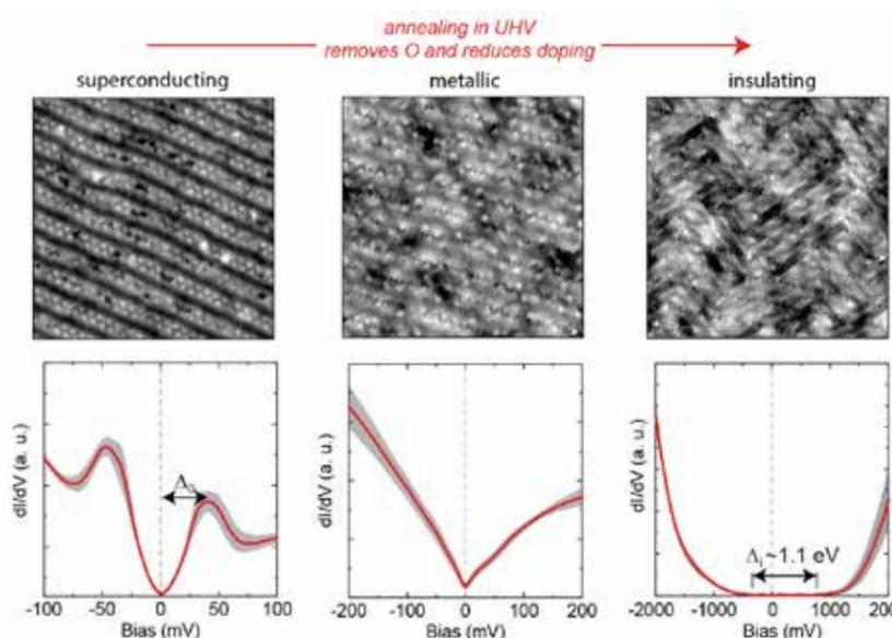
Imaging the evolution of the electronic structure of high- $T_C$  superconductor  $\text{Bi}_2\text{Sr}_2\text{CaCu}_2\text{O}_{8+x}$  as a function of in-situ doping. STM topographs (top row) and average  $dI/dV$  spectra (bottom row) acquired at 4 Kelvin. [Zhao *et al.*, *Nature Materials* (2019).]
