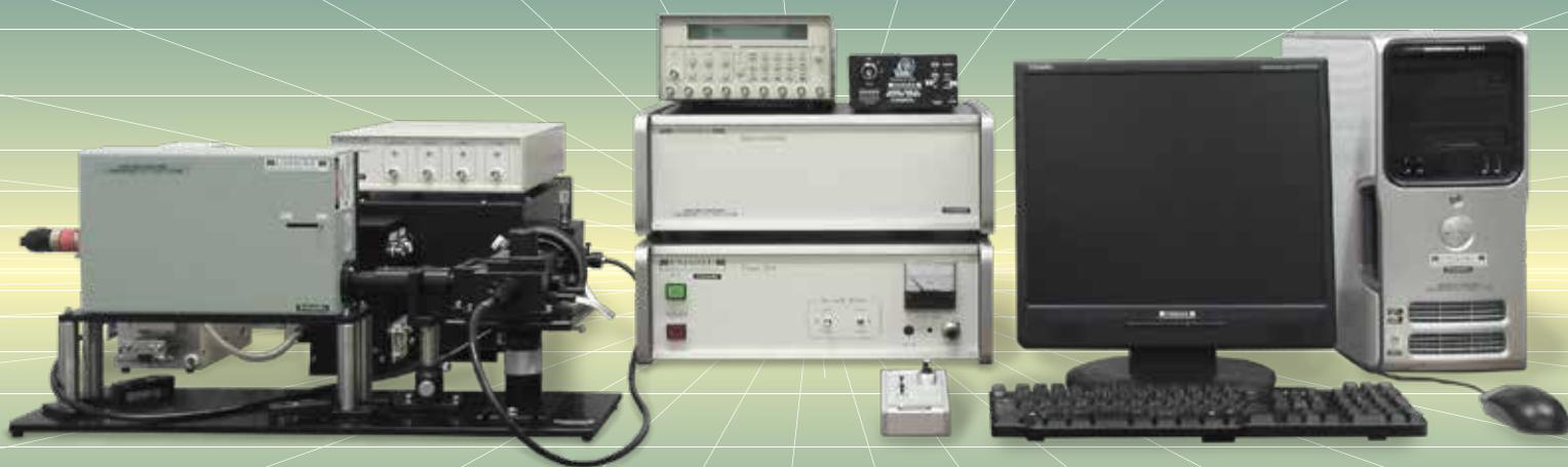
Data are acquired by the combination of a photomultiplier detector and a digital oscilloscope in the single-wavelength monochromator system, and by the combination of a photodiode array detector and a high-speed AD converter in the multi-channel spectrophotometer system. In both systems, time resolution up to 10 nsec is available.
