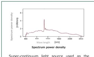
Super-continuum light source used as the probe light source in picoTAS emits light in a broad wavelength range from visible to near-infrared region. Though its light intensity has wavelength dependence, picoTAS can adjust the light intensity automatically which enters into detectors.
