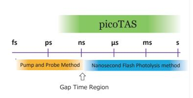
There are mainly two conventional transient absorption (TA) techniques, Pump & Probe method and Nanosecond Flash Photolysis method. However these methods have difficulty in measuring the time region from 1 to 20 nanoseconds in which many important phenomena exist.
