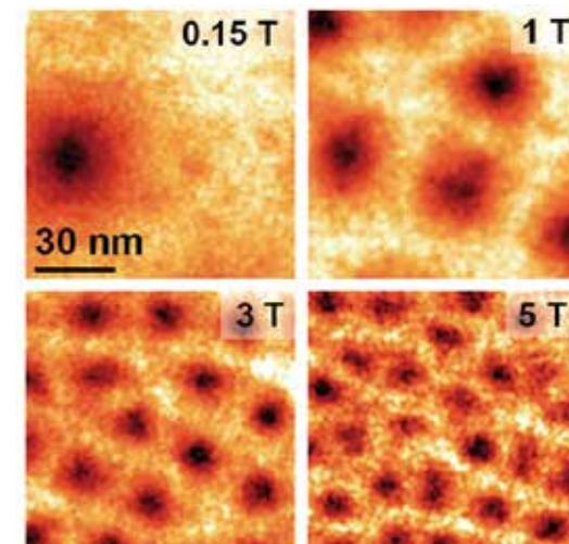
$dI/dV$  maps showing a vortex lattice on the surface of proximitized topological insulator Bi<sub>2</sub>Te<sub>3</sub> thin film grown on a superconductor Fe(Te,Se) [Zhao et al., *Physical Review B* (2018)].
