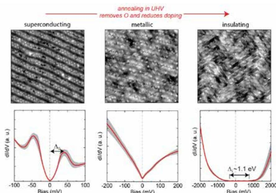
Imaging the evolution of the electronic structure of high- $T_c$  superconductor Bi<sub>2</sub>Sr<sub>2</sub>CaCu<sub>2</sub>O<sub>8+x</sub> as a function of in-situ doping. STM topographs (top row) and average  $dI/dV$  spectra (bottom row) acquired at 4 Kelvin. [Zhao et al., *Nature Materials* (2019).]
