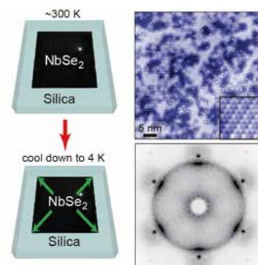
Strain manipulation of a charge density wave in NbSe<sub>2</sub>. STM topograph (top right) and a Fourier transform of a  $dI/dV$  map showing quasiparticle interference (bottom right) [Gao et al., *PNAS* (2018)].
