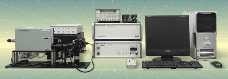
Data are aquired by the combination of a photomultiplier detector and a digital osciloscope in the single-wavelength monochromator system, and by the combination of a photodiode array detector and a high-speed AD converter in the multi-channel spectrophotometer system. In both systems, time resolution up to 10 nsec is available.
