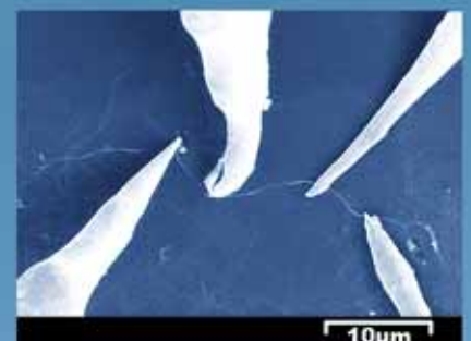
Four probes over carbon nanotube
