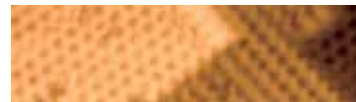
Fig. 2 Temperature: 83K Scan area: 15.5nm X 4.3nm Sample bias: 1.2V Tunnel current: 1.0nA
