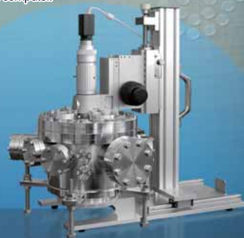
High vacuum 4-probe stage and optical microscope (custom-order)
