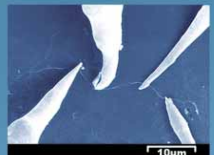
Four probes over carbon nanotube
