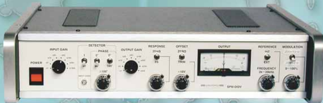
Lock-in Amplifier for KFM Measurement
