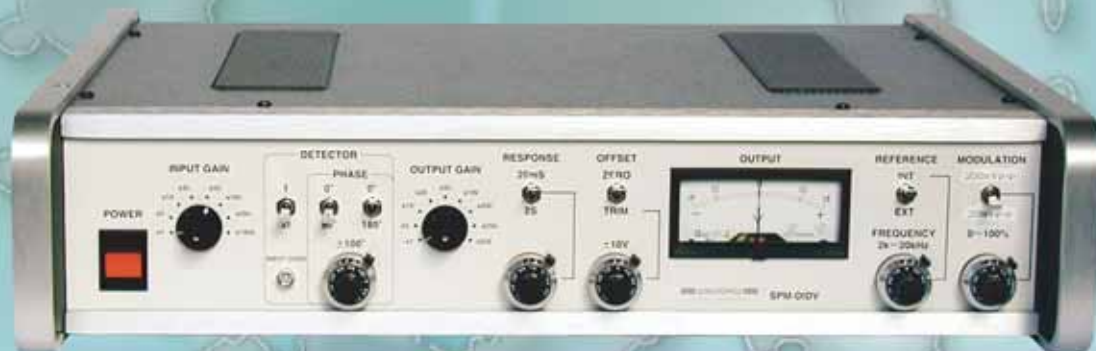
Lock-in Amplifier for KFM Measurement
